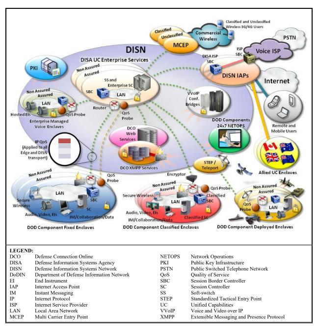
Figure 2-1. Notional DoDIN Network Architecture
